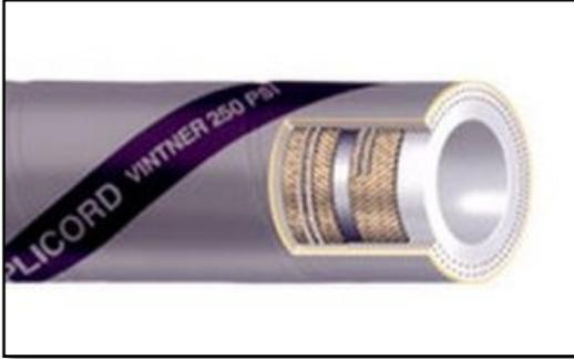
**Application:** For handling in-plant and/or tank truck transfer of wine, beer, potable water and other non-oily, liquid food stuffs.
