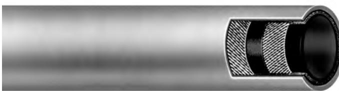
For heavy duty air service in industry and quarries. Oil resistant tube. Oil, weather and abrasion resistant cover. Also available with synthetic fabric braid carcass, at some sacrifice in working pressure.
