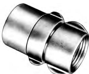
*The use of 3" hose is increasing. By actual test, the temporary restrictions to 2 $\frac{1}{2}$ " waterway for thread does not increase friction loss enough to be noticeable. To use 2 $\frac{1}{2}$ " threads, the coupling is constructed in 5 parts to permit expanding 3" expansion ring in hose bowl with standard 3" expander segments. Furnished pin lug and rocker lug. Complete with expansion rings, swivel and bowl gaskets.*
