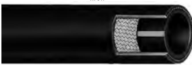
For leaded or unleaded gasoline, and up to 50% aromatic hydrocarbons. Also for use as a Stage II curb pump vapor recovery system hose. 150 PSI working pressure all sizes.
