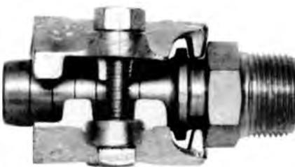
For use with couplings having safety interlock. While clamp compresses hose onto coupling shank, clamp teeth grip grooved collar on the coupling.
