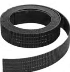
For a great variety of clamping applications. Up to 150 lbs. The gray polypropylene Q-Bands and Q-Clips are non-toxic and ultraviolet resistant. Temperature range is 0° F to + 200° F. Bands are easily tensioned and cut with Q-Gun Hand Tool. Bands are 100 ft long and 1/2" wide.
