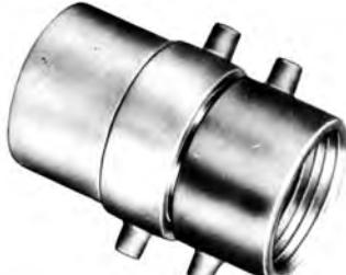
*These medium duty cast brass couplings are manufactured for use with single jacket mill hose not usually subject to more than 400 lbs. surged pressure. Used by industry on both fire and water hose. Available in sizes 1", 1 $\frac{1}{4}$ ", 1 $\frac{1}{2}$ ", 2" and 2 $\frac{1}{2}$ " with pin lug and rocker lug wrenching feature. Furnished complete with expansion rings, swivel and bowl gaskets.*
