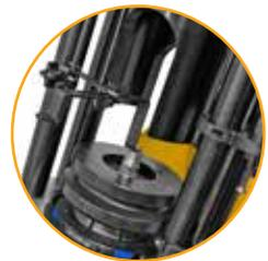
Coupling stop makes repetitive crimps faster by not having to visually align the fitting before each crimp.
