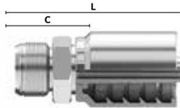
Knowing the overall length of the assembly desired, you subtract the "C" cut-off factor for each fitting from the overall length to obtain the hose cut length.
