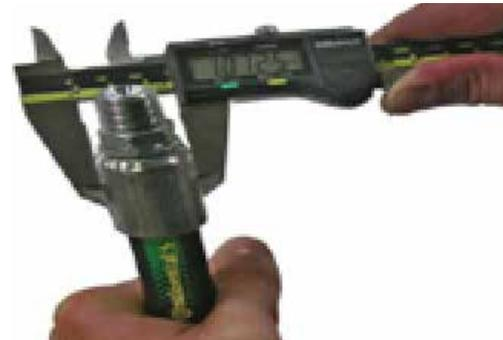
Verify crimp diameter with calipers.
