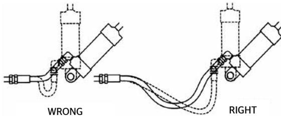
To avoid twisting in hose lines bent in two planes, clamp hose at change of plane, as shown.
