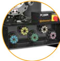
5 die storage pockets panel installed to keep frequently used die sets readily available.
