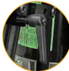
Retraction Stop limits ram retraction for quick repetitive crimps.
