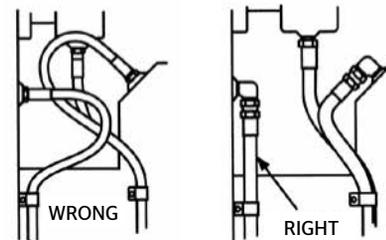
Avoid a sharp twist or bend in the hose by using proper angle adapters compatible with the hose.
