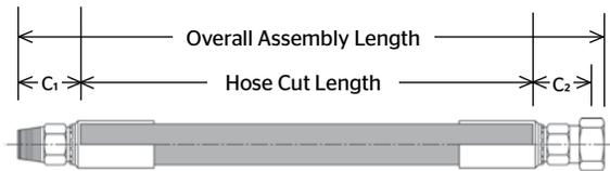
Hose assemblies should be manufactured to the following length tolerances:
