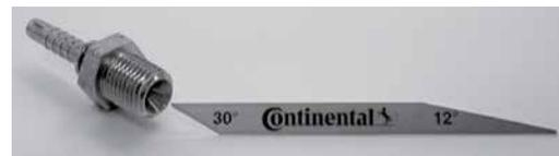
6. Compare measurements above to the tables in the fitting catalog or identification manual to complete the identification of the fitting.
