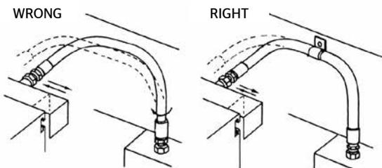
Hose should not be twisted. Hose is weakened when installed in a twisted position. Also, pressure in twisted hose tends to loosen fitting connections. Design is such that the machine motion produces bending rather than twisting.
