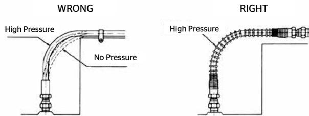
Where the radius falls below the required minimum, an angle adapter should be used as shown on the previous page to avoid sharp bends in the hose.
