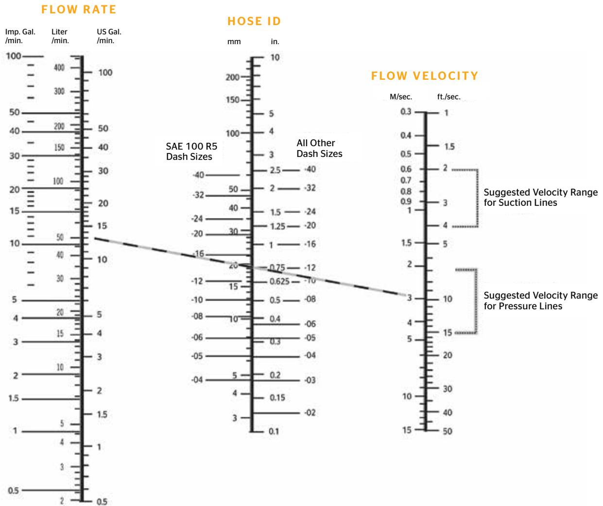
The following table represents the maximum flow rate in gallons per minute (GPM) by Hose ID for pressure lines and suction lines. The recommended maximum fluid velocity for pressure systems is 15 feet per second (FPS).
