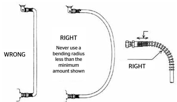
Never use a bending radius less than the minimum shown in the hose specification tables. To reduce collapsing of line and restriction of flow, avoid a sharp bend in the hose by using the proper spring guard. Exceeding minimum bend radius will greatly reduce hose assembly life.
