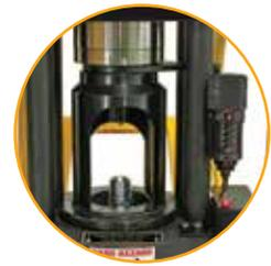
LED indicator light will turn on to indicate that the crimp is complete.
