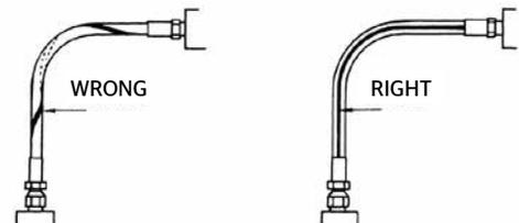
To prevent twisting and distortion, the hose should be bent in the same plane as the motion of the boss to which the hose is connected.
