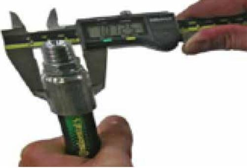
*Verify crimp diameter with calipers.*
