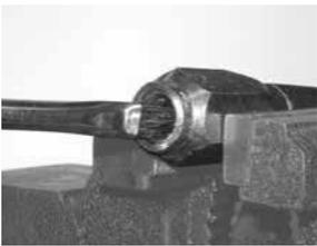
*Apply lubricant to stem and hose tube.*
