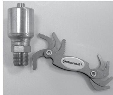
5. Measure the angle of the fitting's sealing surface using the Seat Angle Gauge.
