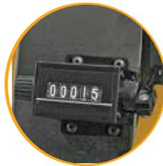
A resettable counter makes it easy to keep track of the number of cuts made.
