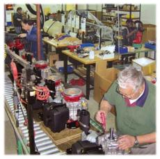
**Riverside Pumps Being Built by Hand**
