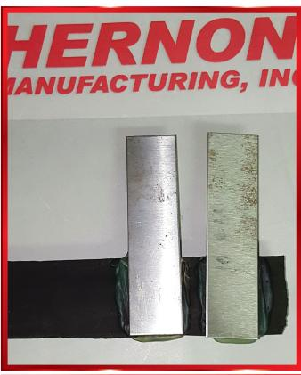
Steel coupons adhered to rubber with Hernon's Fusionbond® 375.
