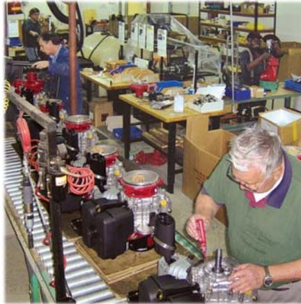
Riverside Pumps Being Built by Hand
